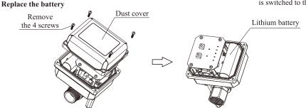
Remove the 4 screws on the dust cover, remove the old lithium battery, replace it with a new one, and insert the plug.
